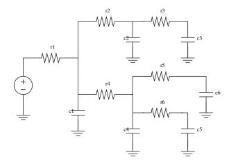
We will use the Elmore delay to model the delay from the source to each of the loads. The Elmore delay to loads 1, 2, and 3 are given by
